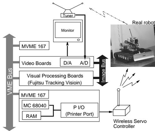
Figure 8: Configuration of the experimental system
