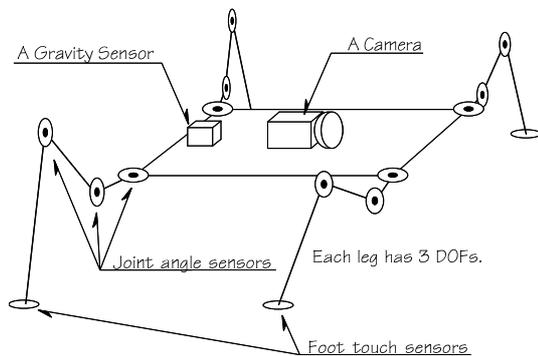
Figure 2: The robot construction
