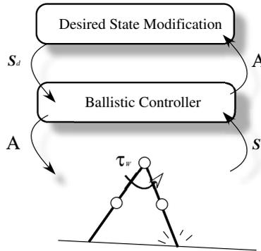
**Figure 1: Proposing layered controller for biped walking**
