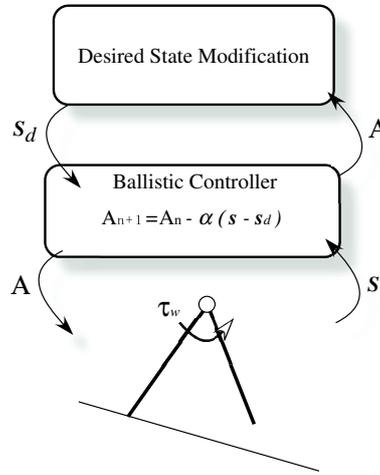
**Figure 3: Layered controller with simple feedback controller**
