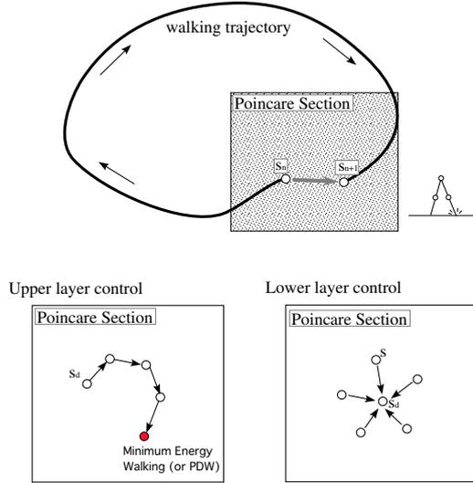
**Figure 2: Poincaré section is taken at heel strike. On this plane, the lower layer of the controller tries to keep the state at heel contact in the same area as the desired one which is given by the upper layer. The upper layer of the controller tries to search the desired state which realize walking mode with minimum energy.**
