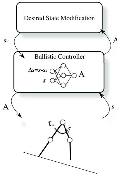
Figure 5: Layered controller with neural network
