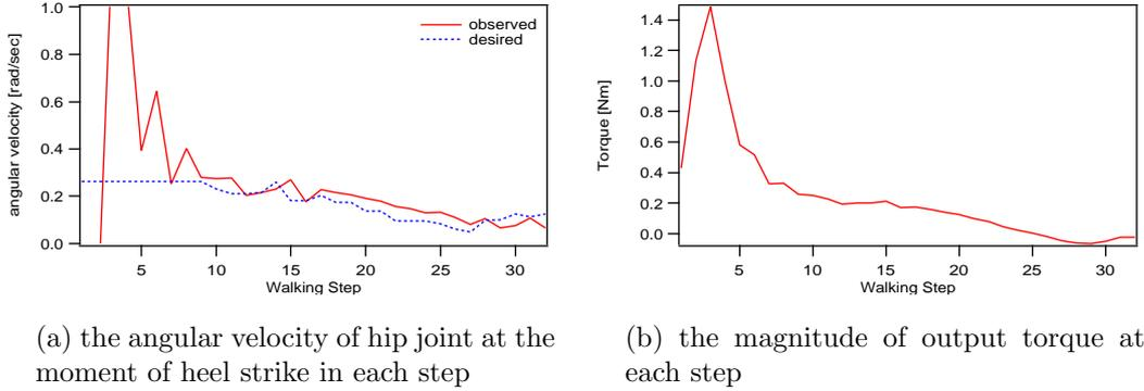
**Figure 4: Walking mode converges to PDW under the proposing controller when the slope is inclined 1 [deg]**
