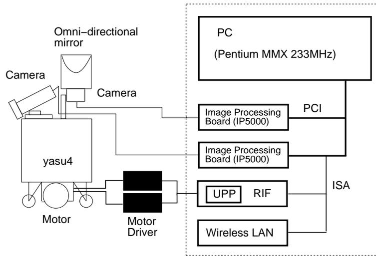
Figure 5.17: An overview of the robot system
