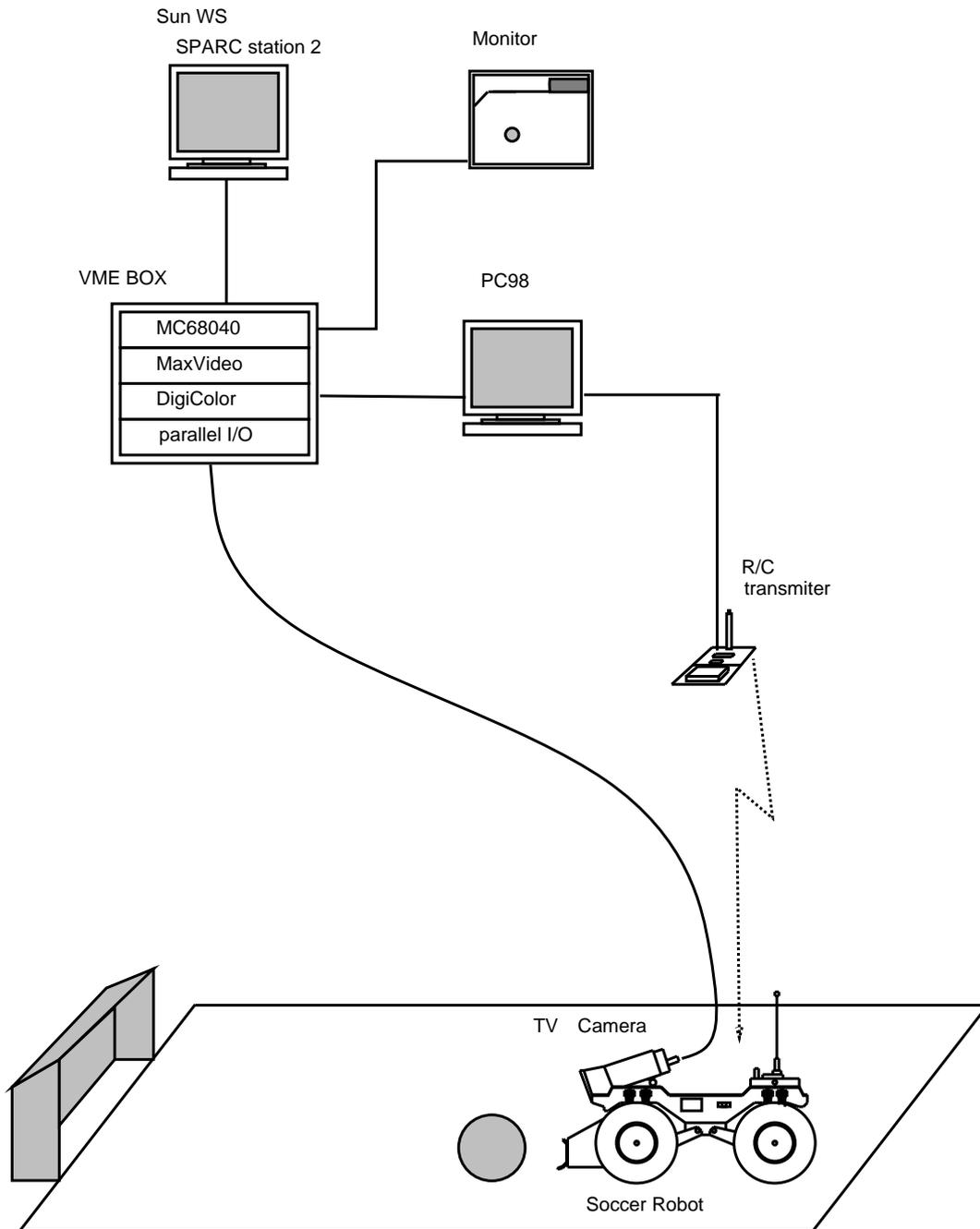
Figure 3.15: A configuration of the real robot
