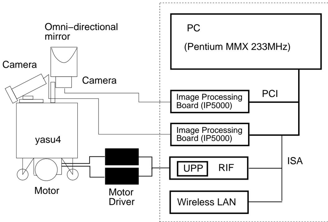
Figure 4.6: An overview of the robot system
