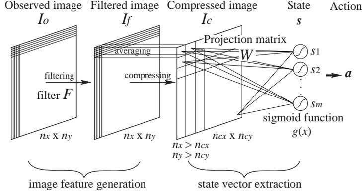
Fig. 1. Image feature generation and action selection model.
