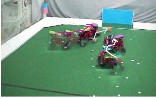
Figure 10: A sequence of the robots' movements using a subjective map in case 2 with large error for robot B.
