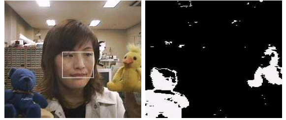
(b) the left camera image of the robot (left: the detected result of the caregiver's face by template matching, right: the detected result of the bright colors)
