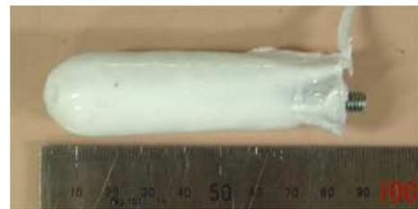
Fig.2 The soft finger-tip with tactile sensors
