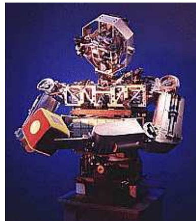
(b) Cog has twenty-one degrees of freedom and various sensory systems.
