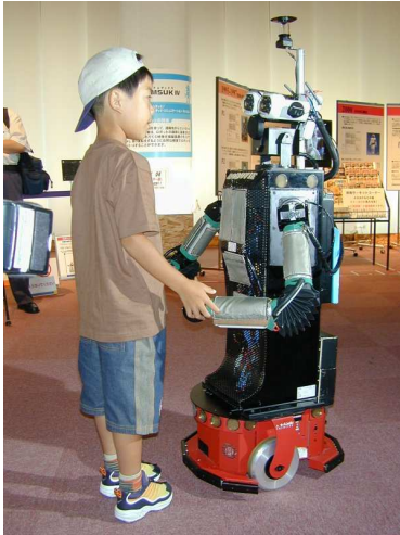
(a) Robovie, an human-like mobile robot that is 120 [cm] tall and has several actuators and sensors.
