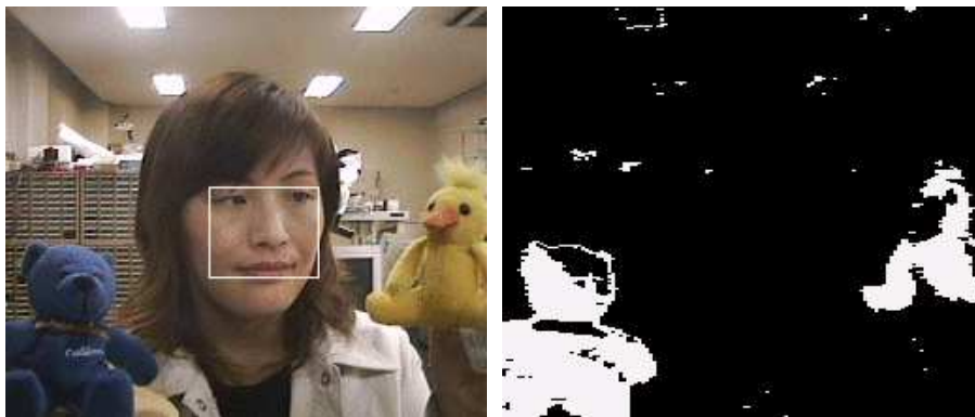
(b) The robot's camera image acquired in the situation (a). The rectangle in the left image shows the position of the caregiver's face detected by template matching, and the highlighted areas in the right show the objects with a bright color extracted by using thresholds in a color space. This processing is conducted by the salient feature detector in the proposed model.
