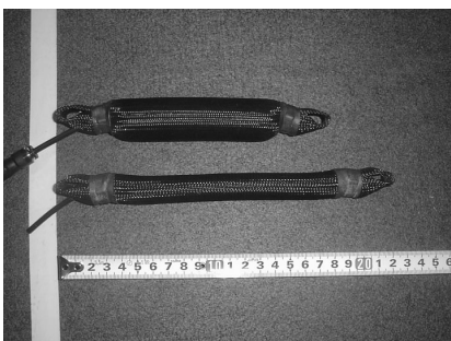
Figure 1: A McKibben type actuator. When the air is supplied into inner tube, it is shrunk (upper), and extend when the air is exhausted (bottom).
