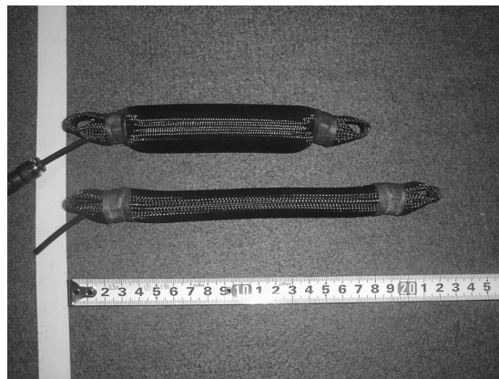
Fig. 1. A McKibben type actuator. When the air is supplied into inner tube, it is shrunk (upper), and extend when the air is exhausted (bottom).
