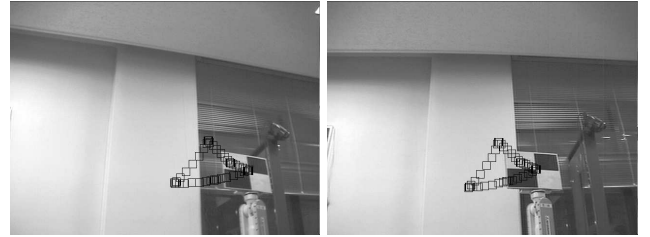
Fig. 10 The learner's view observing the demonstration: the demonstrator's trajectory of the end-effector.
