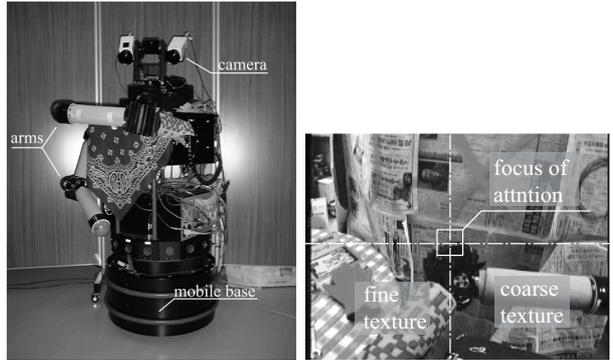
(a) The robotic test-bed (b) An egocentric view of the robot
