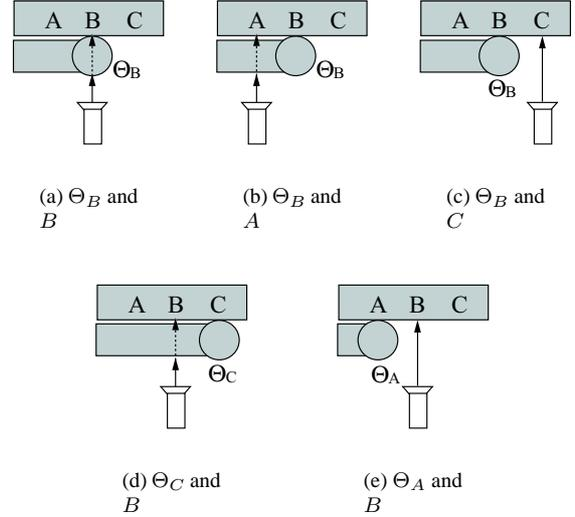
**Figure 4. Five simplified situations in the robot exploration: A top rectangle indicates the robot's trunk while a rectangle with a circle in the middle indicates the robot's arm that has a sliding DoF in the horizontal axis. The bottom object shows the posture of the robot's camera head while the arrow indicates its focus of attention. Notations correspond to those in Fig. 3.**
