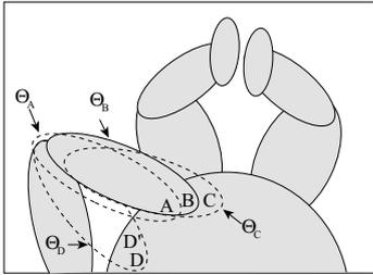
**Figure 3. An example of self-watching view of the robot in double-touching: three ellipsoids with solid and broken lines are links in the postures ( $\Theta_A$ ,  $\Theta_B$ , and  $\Theta_C$ ) by which it touches with the parts labeled  $A$ ,  $B$ , and  $C$ , respectively. The rest ellipsoid with the symbols  $D$  and  $D'$  is one in the posture ( $\Theta_D$ ) by which it touches the part labeled  $D$  with occlusion at  $D$  and  $D'$ .**
