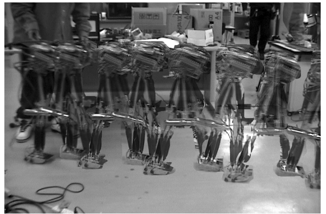
第 6 図 A motion sequence of walking of the 3D pneumatic driven walker
