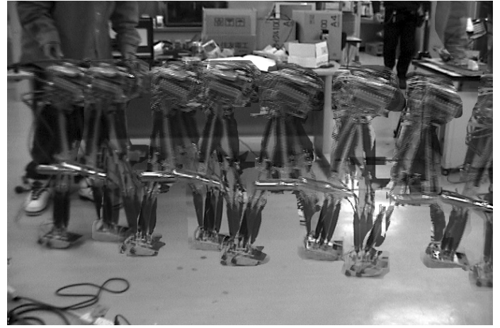
Fig. 10. A motion sequence of walking of the 3D pneumatic driven walker
