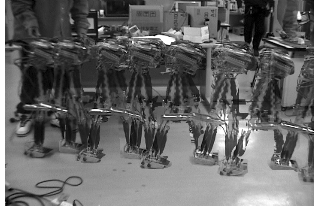
Fig. 5. A walking sequence of the developed biped with proposed control
