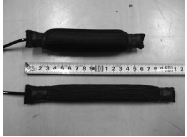
Fig. 3. McKibben artificial muscles by Hitachi Medical Corporation. When it contracts, its diameter becomes 20 [mm]. It generates 800 [N] when it is supplied with 0.7 [MPa] pressure.
