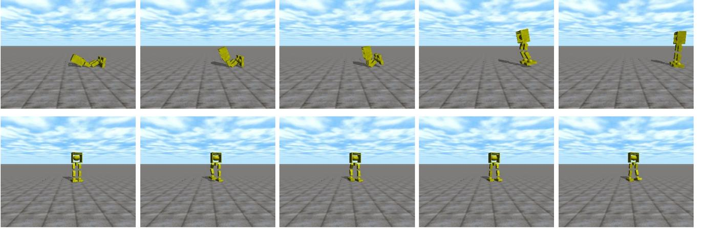
Fig. 3. Simulation results for three variant types of robots: First row shows an actuated biped robot with 3 degrees of freedom per leg and an actuated gyro (close loop control). The second row shows the same robot walking using an open loop control for the legs.
