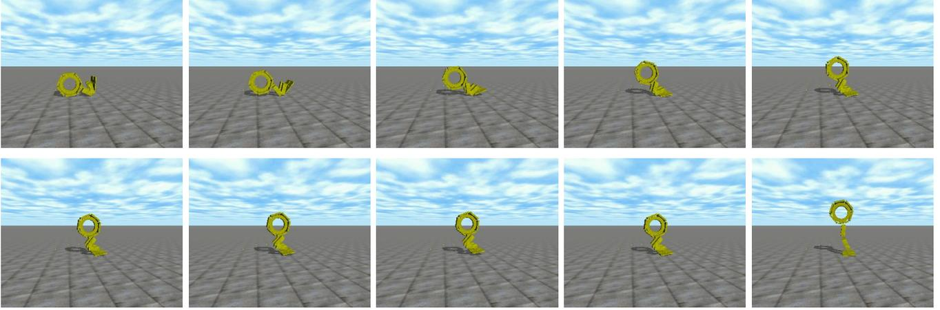
Fig. 5. Biped with realistic specifications of a motor/brake combination standing up.
