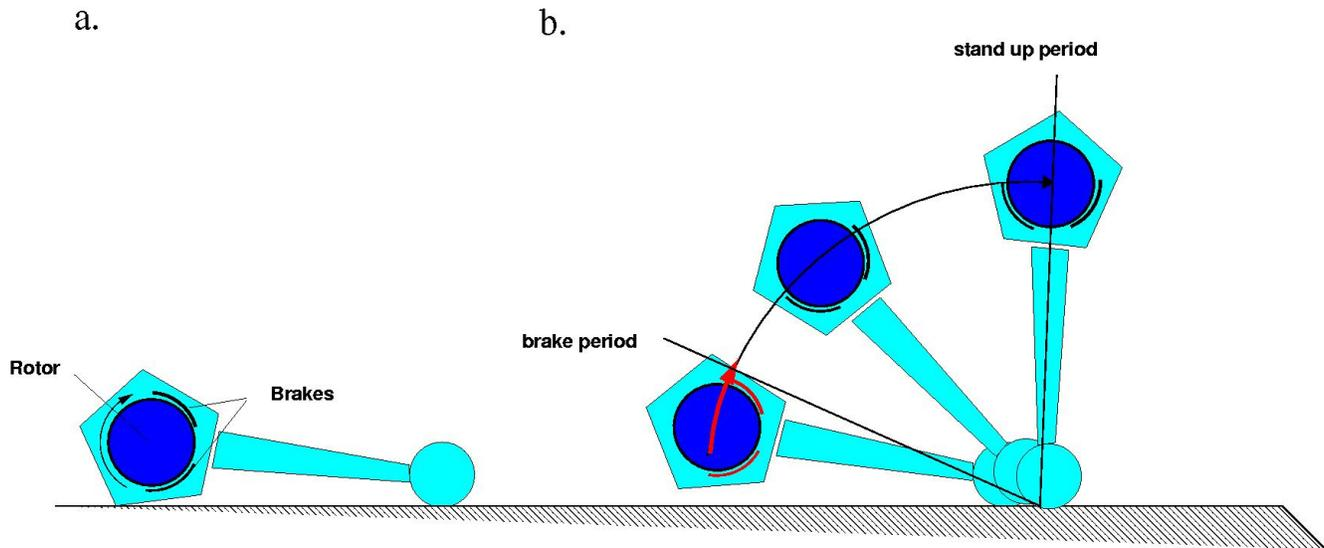
Fig. 4. A robot during standup: a. The robot is prepared by accelerating the rotor in the direction of the desired movement of the robot. In this way the needed momentum is stored in the rotor. b. The rotor is stopped by braking and the robot stands up.
