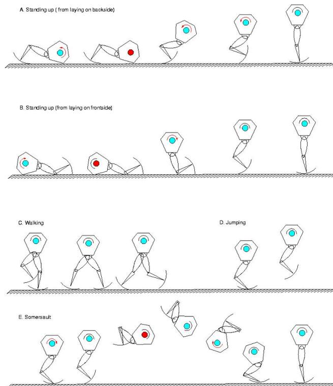
Fig. 7. Hypothetical actions that can be controlled with the rotor/ brake mechanism. A red rotor indicates that the brake is activated.
