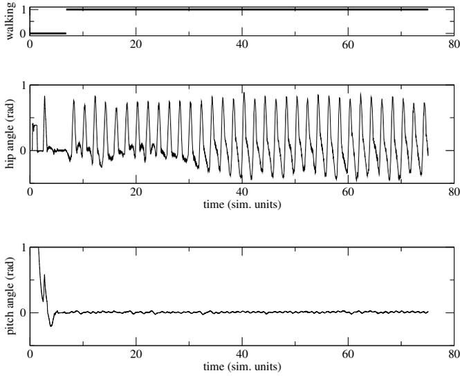
Fig. 2. Motion patterns of walking in the actuated biped robot. On top: the state of the waling behavior. Middle: Motion pattern of the left hip. The motion pattern is not entirely regular. Below: The state of the pitch value ( $\alpha$ ). A small oscillation can be seen.
