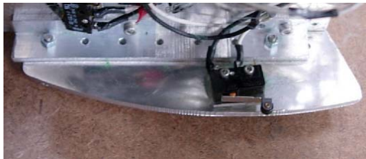
Fig.3 Robot Sole : The radius of the foot is 220[mm]. ON/OFF switches are attached on both side of soles to detect a heel strike.
