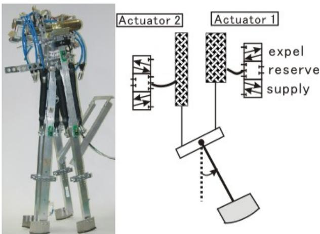
**Figure 1:** The biped driven by the pneumatic muscles “Que-kaku” (left) and the schematic construction of the joint driven by the antagonistic pair of muscles (right).
