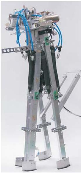
Fig. 1 A 2D biped walker with McKibben pneumatic actuators. The robot is self-contained and has two air bottles with regulators, three-position air valves, a microcomputer board, and an electrical battery.
