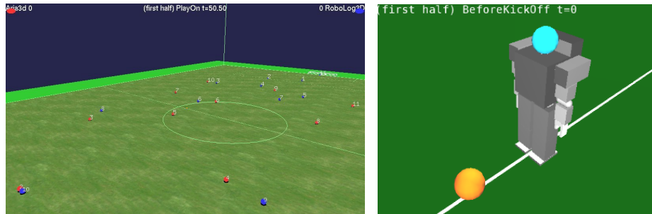
Fig. 2. (Left) The first simulation: 11 vs 11 spheres with omni-drive and kick effector. (Right) The first humanoid model based on the HOAP-2 robot from Fujitsu.
