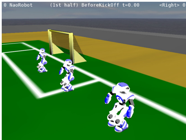
Fig. 3. A screen shot of the NAO soccer simulation in Simspark as used in the 3D Soccer Simulation League at RoboCup 2008.
