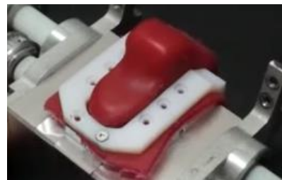
Fig. 8 Deformation of the tongue made of soft material by the tongue blade linkage
