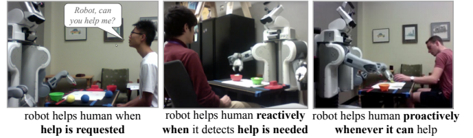
Fig. 1. Different initiative models for robot assistance during collaborative task executions: human-initiated help (left), robot-initiated reactive help (middle), and robot-initiated proactive help (right).
