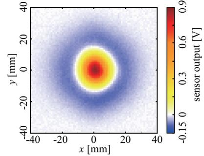
Fig. 2. Difference of Gaussian like spatial response of the proposed sensor with one magnet located at the origin.
