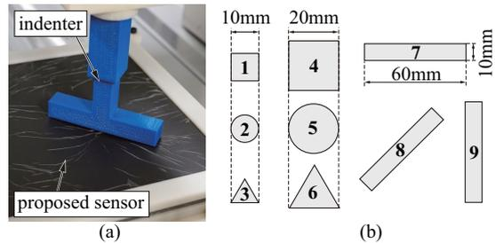
Fig. 4. Experimental setup. Nine types of objects were pressed onto the sensor surface with 5 mm depth. (a) Appearance of the setup. (b) Bottom shape of the nine objects used in this study. Objects 7, 8, and 9 had the same rectangular shape but different angles against the  $x$ -axis.
