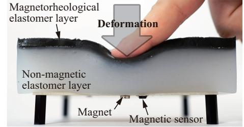
Fig. 1. Appearance and structure of the proposed tactile sensor that can detect applied depth directional deformation as a change of magnetic field.
