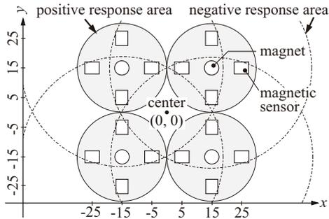
Fig. 3. Arrangement of 4 magnets and 16 magnetic sensors on  $x$ - $y$  plane.
