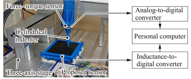
Fig. 2. Experimental setup for measuring the sensor response curves. A normal force was applied to the sensor surface by a three-axis robot stage with a cylindrical indenter. A personal computer captured the inductance and the outputs of a force-torque sensor via an inductance-to-digital converter and analog-to-digital converter.
