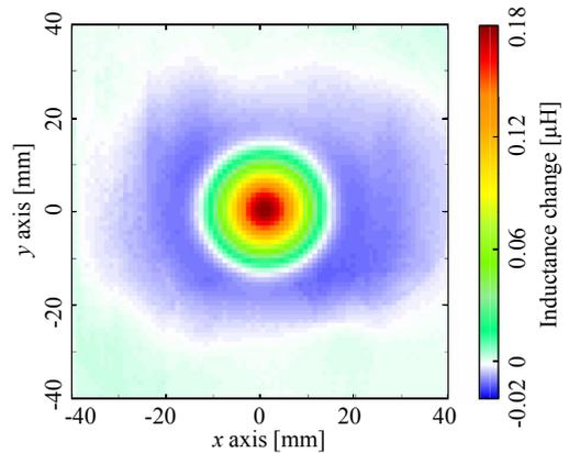
Fig. 5. Spatial response of the sensor with a type A inductor. The color indicates that the inductance changed from its initial value.
