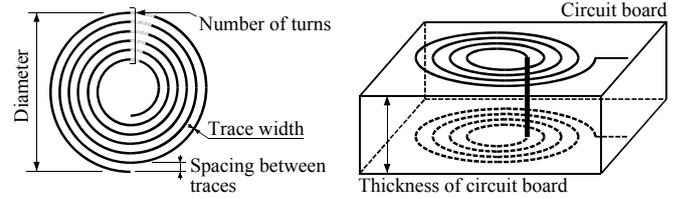
Fig. 3. Inductor parameters of a two-layer planar spiral inductor printed on both surface of a rigid circuit board.
