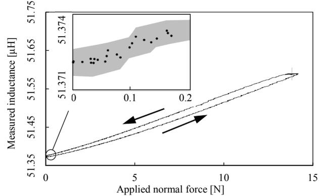
Fig. 4. Measured sensor response curves versus the applied normal force across 10 trials. The inset shows a magnification of the initial part of the curve. The solid line and dots indicate the mean value of the inductance, and the arrows depict the direction of the applied normal force. The shaded region indicates twice the standard deviation ( $2\sigma$ ) of the inductance.
