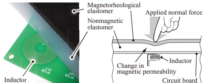
Fig. 1. Appearance of the proposed sensor and its cross-sectional schematic. An inductor is printed on a circuit board while magnetorheological and nonmagnetic base elastomers cover the board.
