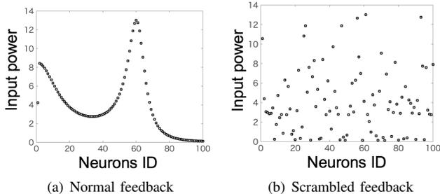
Fig. 3. Coding examples of a sound for the auditory feedback. The model converts the vocalized sound into its frequency spectrum. In the case of normal auditory feedback (a), a power in each frequency band is fed to a neuron. This correspondence between the band and the neuron is unchangeable. In contrast, the neurons that receive the input are randomly selected every time in the scrambled feedback (b).
